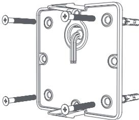
**2** Push through mounting holes and produce marks on the wall intended for installation. Note that the cable entry must be at the top. Use min. 2 including screws to secure the bottom part of housing to the installation location.
